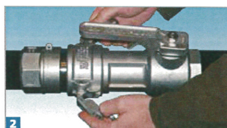
2 Cam Arms Lock Coupler and Adaptor Together
