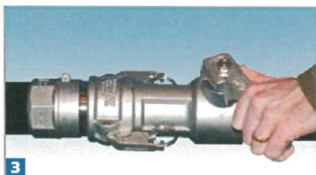
3 Locking Handle Opens Valves
